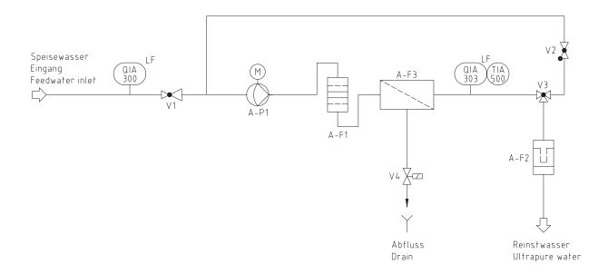
A-F1 Filter cartridge A-F2 Sterile filter
