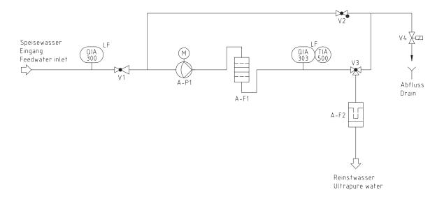
A-F1 Filter cartridge A-F2 Sterile filter A-P1 Circulation pump **QIA 300** Feedwater conductivity **QIA 303** Ultrapure water conductivity TIA 500 Temperature sensor V1 Pressure reducer V2 Check valve V3 Dispensing valve V4 Solenoid rinsing valve
