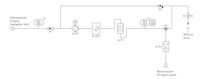
A-F1 Filter cartridge A-F2 Sterile filter A-P1 Circulation pump UV-photooxidation A-UV1 **QIA 300** Feedwater conductivity QIA 303 Ultrapure water conductivity TIA 500 Temperature sensor Pressure reducer V1 V2 Check valve V3 Dispensing valve V4 Solenoid rinsing valve
