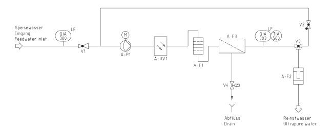
A-F1 Filter cartridge A-F2 Sterile filter
